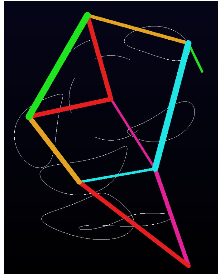
Fig. 20 Motion trajectory of centers of gravity of individual members of the Jansen's linkage
